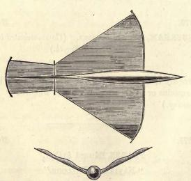
An elongated body pointed at both ends contains the requisite machinery and the passengers.
